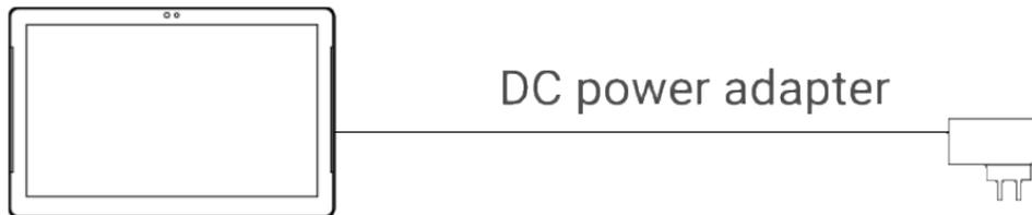
Requires a 3.5 x 1.35mm barrel jack connector with the following configuration
