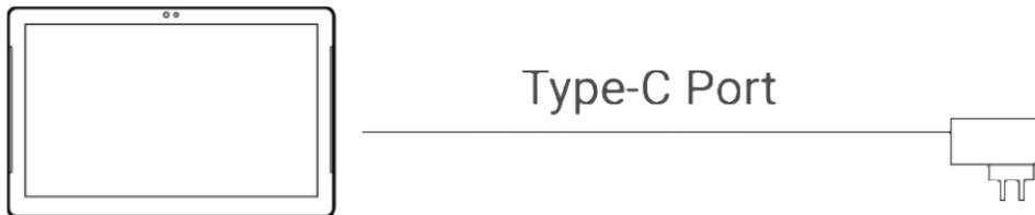
Requires a USB type C connection providing 5Vdc and at least 2A. This can be a dedicated USB power supply unit or another device powering the screen with at least the 2A required
