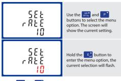
Use the and P buttons to choose the desired pulse rate. To save the new setting, hold the button for 3 seconds until the selection stops flashing.
