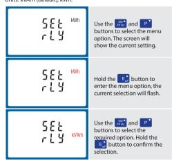
Hold the WA button for 3 seconds to exit the set up menu.
