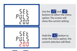
Use the properties and by buttons to choose the desired pulse rate. To save the new setting, hold the button for 3 seconds until the selection stops flashing.
