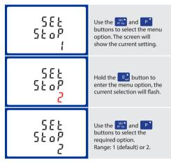
On completion of the entry procedure, hold the button for 3 seconds until the selection stops flashing.
