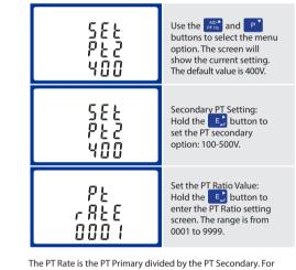
Example: Voltage Transformer - 11000+110=100, so the PT Rate would be 0100 and the PT2 would be 110.
