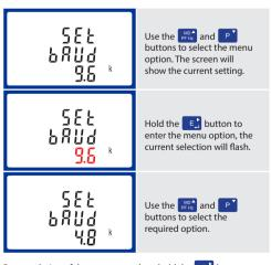
On completion of the entry procedure, hold the  $\begin{tabular}{c} E_{\bullet} \end{tabular}$  button to confirm the setting.
