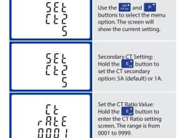
The CT Rate is the CT Primary divided by the CT Secondary. For Example: 200/5A Current Transformers - 200÷5=40, so the CT Rate would be 0040 and the CT2 would be 5.
