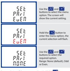
On completion of the entry procedure, hold the button for 3 seconds until the selection stops flashing.
