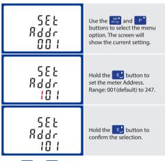
Use the wind and P buttons to choose the necessary number, then press the button to move along to the next number. To save the new setting, hold the button for 3 seconds until the selection stops flashing.
